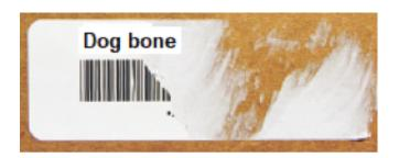
A general-purpose hot melt adhesive with excellent quickstick properties. This adhesive exhibit excellent adhesion to a broad range of packaging surfaces and has improved die cutting and stripping attributes compared to other hot melt rubber-based adhesives. Product handles without tearing until applied. After being applied it has immediate tack, no set up time. Product is strong and durable but destructible after being applied.
